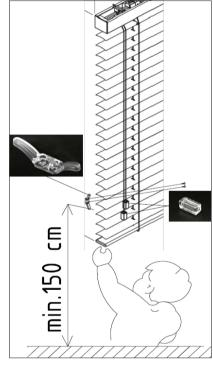
Endings of operation cords were finished with PVC elements (cord endings) to prevent the cords from twisting and creating a loop.
